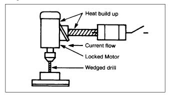
Instead of continuing to draw normal motor load current, the locked drill motor shaft causes the motor to draw "Locked Rotor Current" which is about six times the normal load current.
