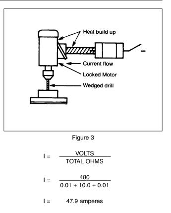
The Figure 3 value of "**overload**" current may be up to about 10 times the normal current value of 47.9 amperes.
